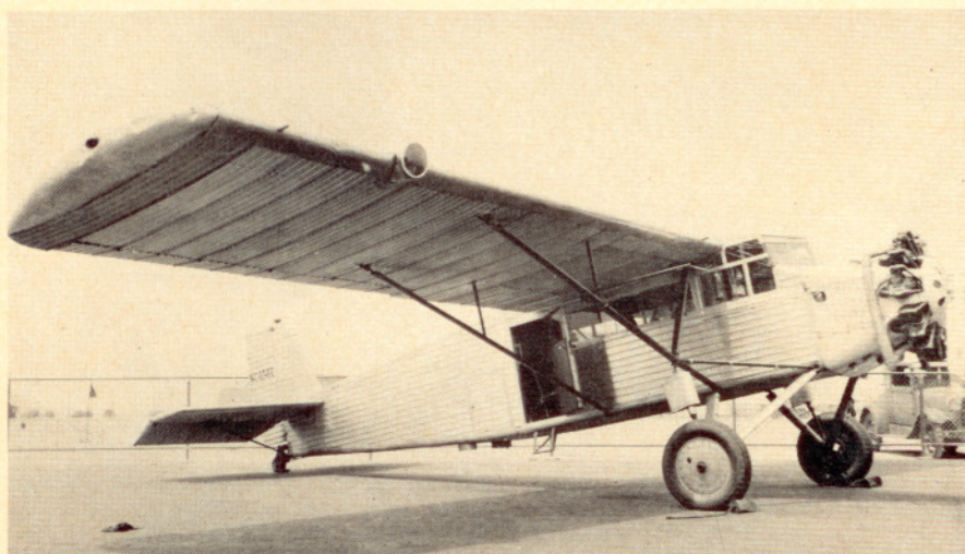
The passenger and baggage compartment doors were on the right-hand side of the Flamingo, while the pilots had a separate door on the left side. Note the fixed landing light on the wing.
