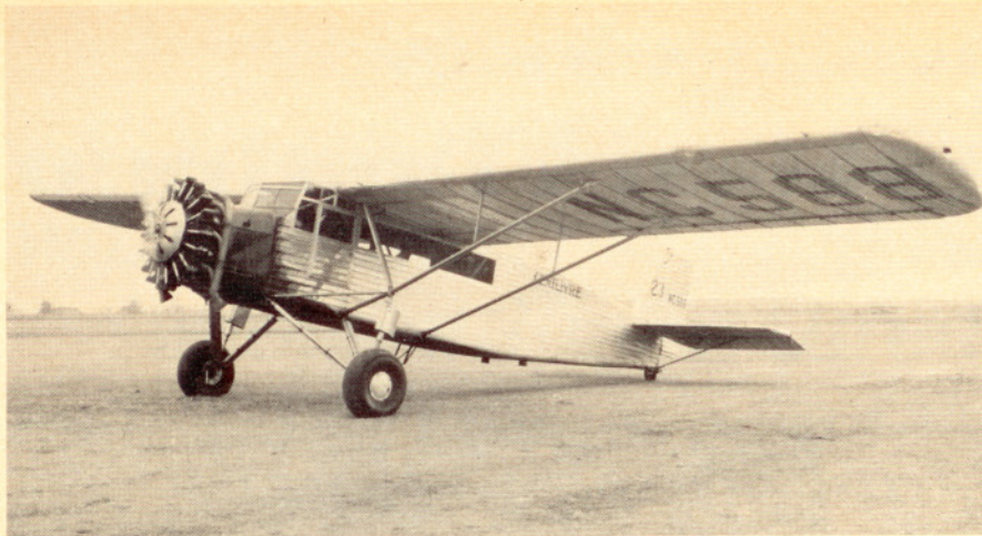
The principal innovation of the Flamingo was the substitution of corrugated sheet aluminum for fabric on an otherwise conventional airframe. Note that the corrugations are only on the outer side of the skin, not alternating as on the contemporary Ford trimotors.
